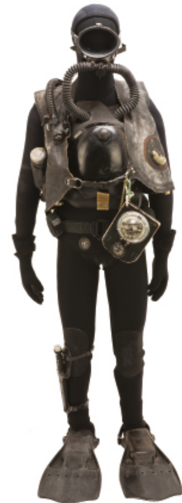
24. Complete diving suit equipped with CO2 oxygen cylinders, from the SDECE Action Service
