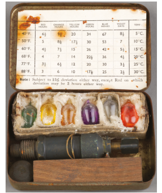
23. AC Delay Mk 1 SOE in its box with acetone ampoules and chemical delay igniter
