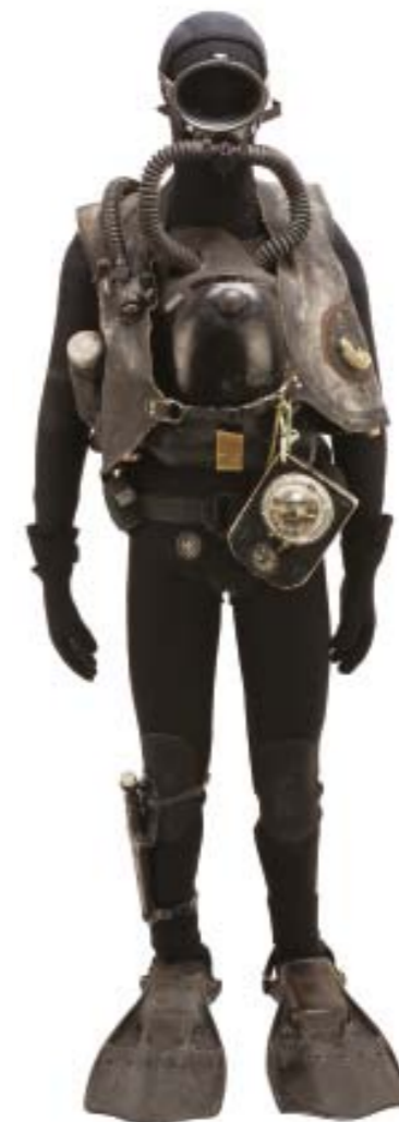
24. Complete diving suit equipped with CO2 oxygen cylinders, from the SDECE Action Service
